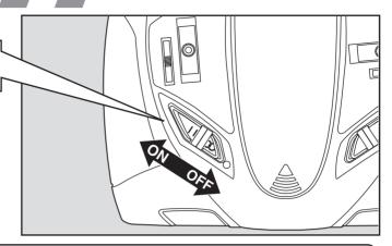
If the power switches are turned off in the opposite order the model may unexpectedly run out of control and cause a very dangerous situation.
