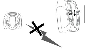
For the engine car, link the transmitter and the receiver at braking position.
