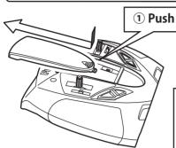
(2) Remove the battery cover from the transmitter by sliding it to the direction of the arrow in the figure.
