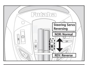
Change the direction of the steering reversing switch.
