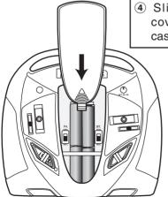
4 Slide the battery cover top onto the case.
