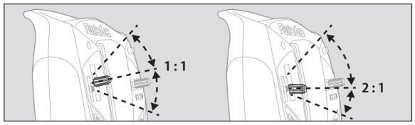
Change the neutral position only when large forward stroke of the throttle stick is need when using an FET E.S.C., etc.
